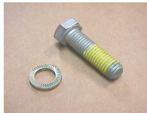
Illustration 2 – New Nordlock and New Halfshaft Bolt
