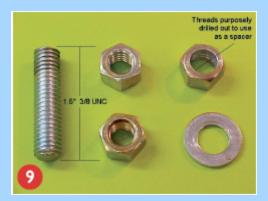
Picture 9 – Parts for Temporary Install Picture 9 shows the parts that Bob used. Bob used a short piece of threaded rod (all-thread) as a stud to replace the bolt. He hand-threaded the stud into the battery, being careful not to over tighten it. Next he took a nut and drilled the threads out such that the nut would slip over the stud. A larger nut would also work, but it would have deformed the plastic cover on the cable terminal.
